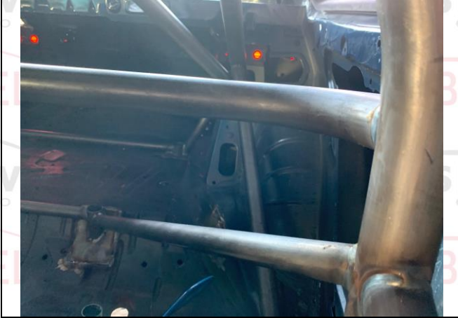
PHOTO 12 SHOULDER HARNESS ATTACHMENT - DRIVER
