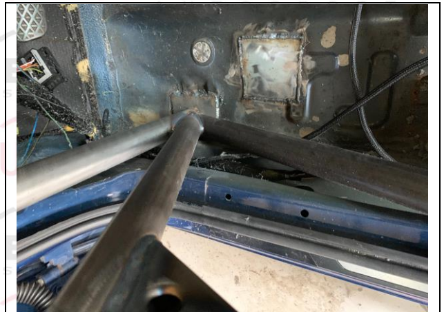
PHOTO 6 FRONT ROLLBAR TO FLOOR ATTACHMENT
