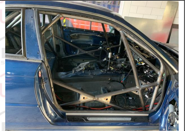
PHOTO 11 ANTI-INTRUSION DOORBAR – CO-DRIVER
