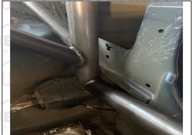
PHOTO 4 MAIN ROLLBAR TO FLOOR ATTACHMENT
